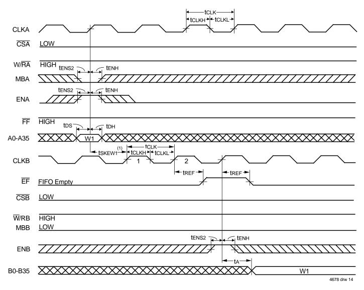
Figure 12. EF Flag Timing and First Data Read when FIFO is Empty (IDT Standard Mode)
