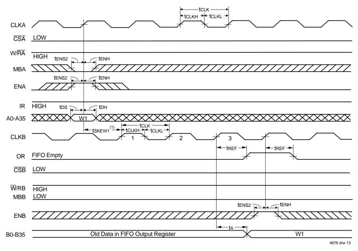
Figure 11. OR Flag Timing and First Data Word Fall Through when FIFO is Empty (FWFT Mode)
