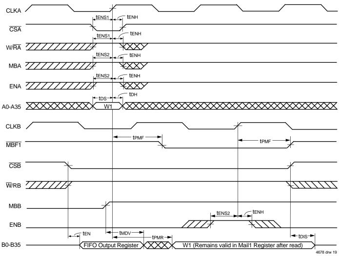
Figure 17. Timing for Mail1 Register and MBF1 Flag (IDT Standard and FWFT Modes)
