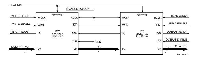
Figure 20. Block Diagram of 32,768 x 9 and 65,536 x 9 Depth Expansion
