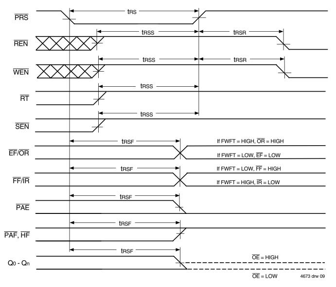
Figure 6. Partial Reset Timing
