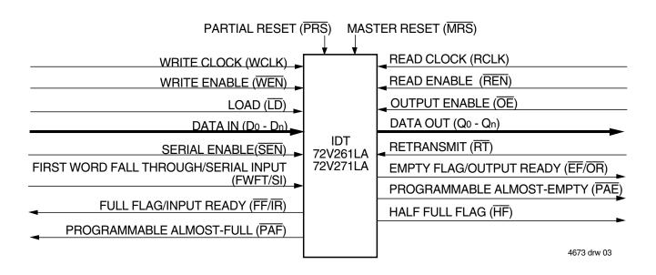
Figure 1. Block Diagram of Single 16,384 x 9 and 32,768 x 9 Synchronous FIFO
