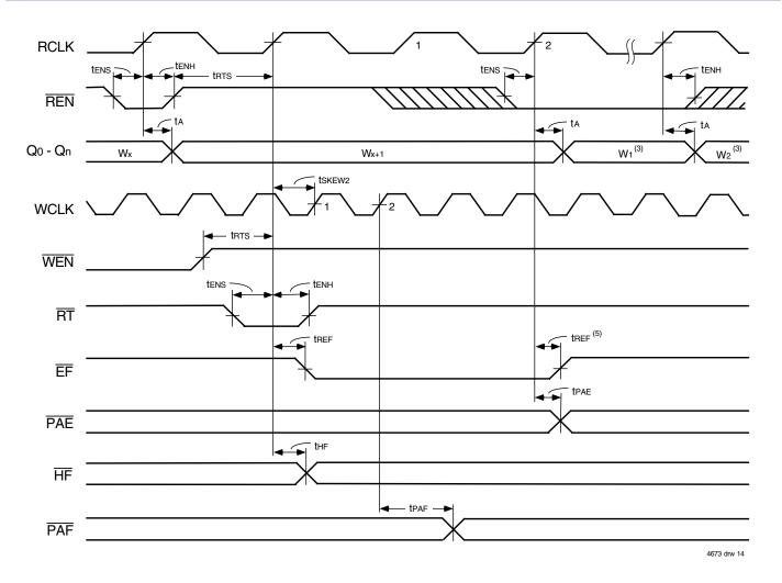
Figure 11. Retransmit Timing (IDT Standard Mode)
