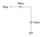
Reset gate clock equivalent circuit
