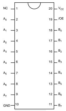
Figure 2. Pin Configuration
