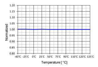
Figure 15. Maximum Duty Ratio (D<sub>MAX</sub>) vs. T<sub>A</sub>
