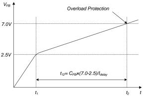
Figure 21. Overload Protection
