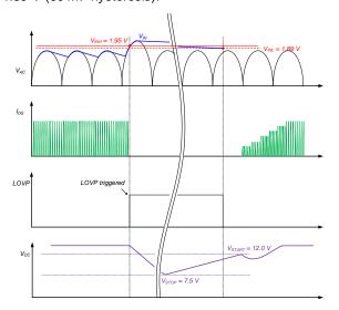
Figure 24. Line Over-Voltage Protection
