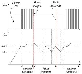
Figure 20. Auto-Restart Protection Waveforms
