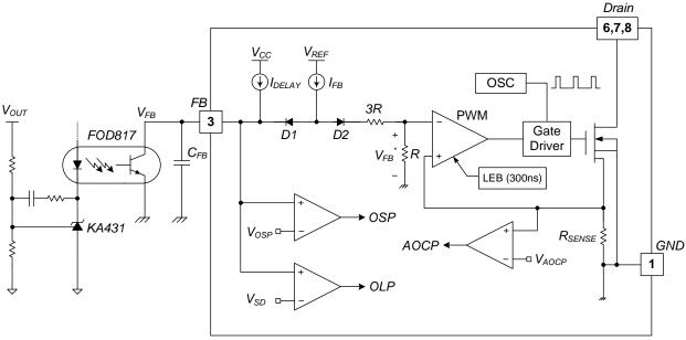
Figure 19. Pulse Width Modulation Circuit
