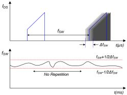
Figure 26. Random Frequency Fluctuation
