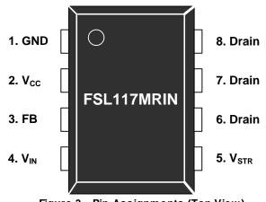
Figure 3. Pin Assignments (Top View)
