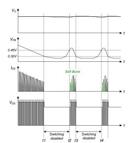
Figure 25. Burst-Mode Operation
