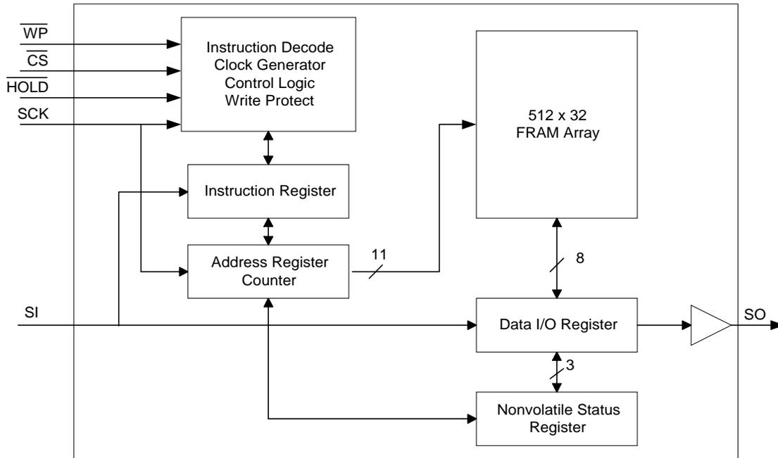
Figure 1. Block Diagram
