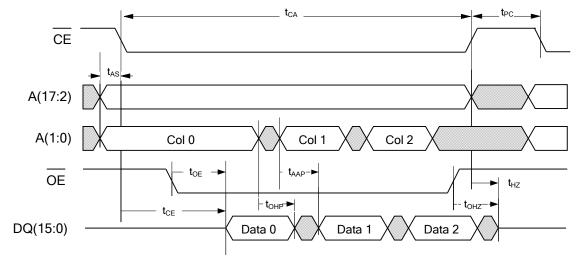
Although sequential column addressing is shown, it is not required.
