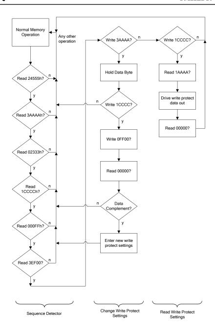
Figure 2. Write-Protect State Machine
