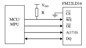
Figure 3. Use of Pullup Resistor on /WE
