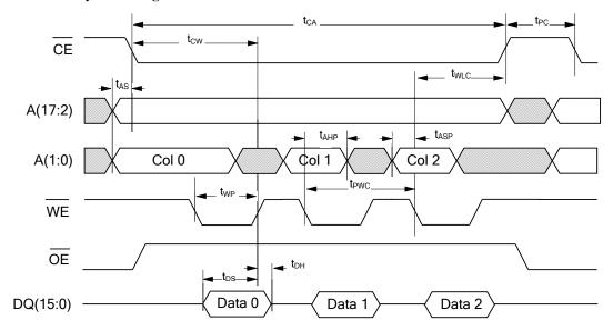
Although sequential column addressing is shown, it is not required.
