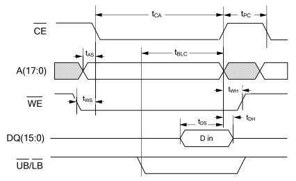
Write Cycle Timing 3 (/CE low) Note: /OE (not shown) is low only to show effect of /WE on DQ pins
