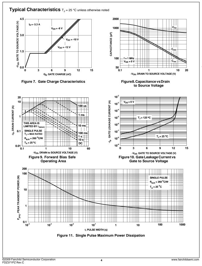
FDZ371PZ P-Channel 1.5 V Specified PowerTrench<sup>®</sup> Thin WL-CSP MOSFET
