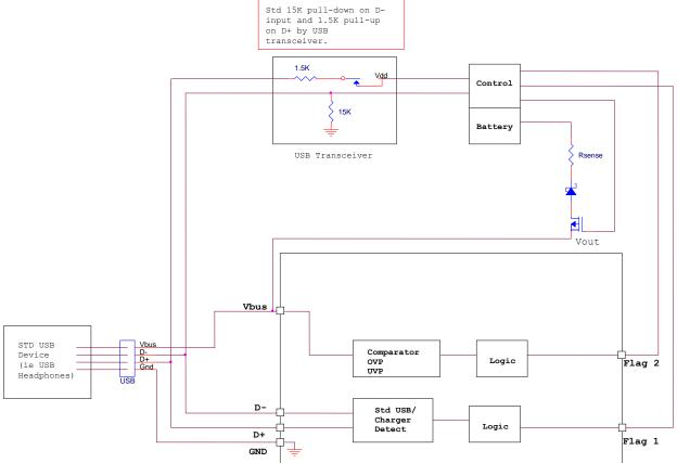
Figure 7. Typical Application System with USB Transceiver
