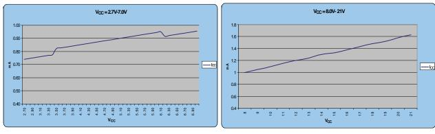
Figure 3. I<sub>BUS</sub> vs. v<sub>BUS</sub> (2.7 V-7.0 V) No Load
