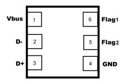
Figure 2. Pin Configuration (Top View)
