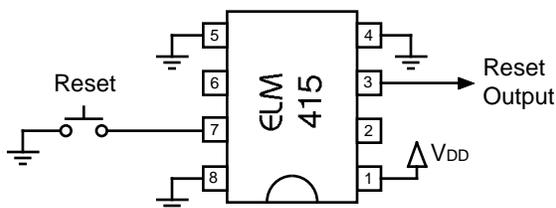
Figure 4. Manual reset circuit
