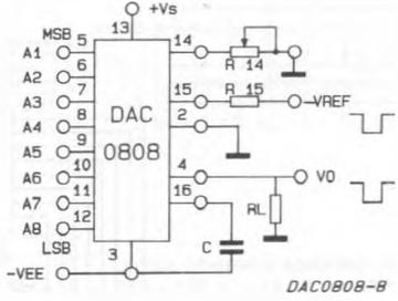
FIGURE 14. Reference Current Slew Rate Measurement
