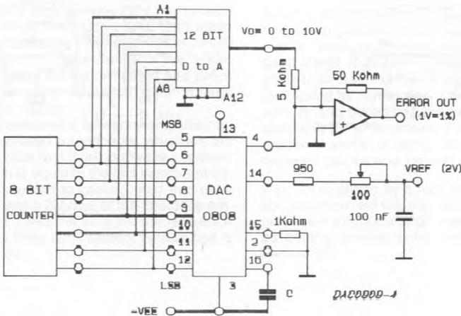
FIGURE 11. Transient Response and Settling Time
