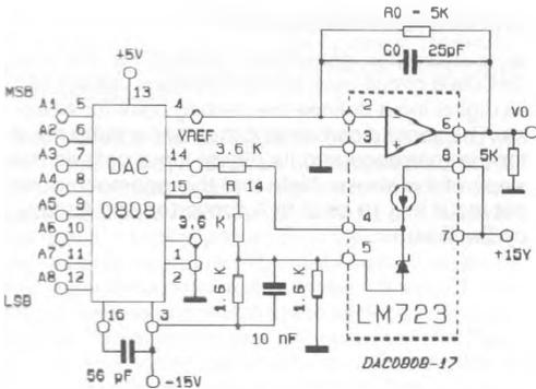
FIGURE 15. Programmable Gain Amplifier or Digital Attenuator Circuit
