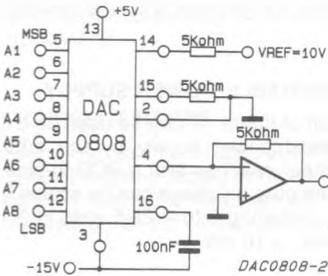
FIGURE 17. Combined output amplifier and voltage reference circuit
