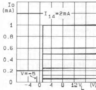
Fig. 6 - Output Voltage Compliance
