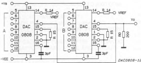
$$V_o = -I_{O1} R_o = \frac{V_{ref}}{R_{141}} |A| R_o$$
