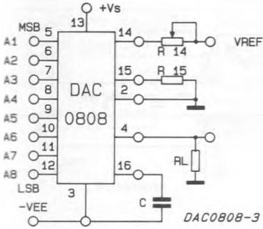
The resistor tied to pin 15 is to temperature compensate the bias current and may not be necessary for all applications.
