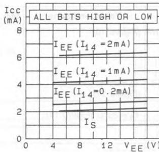
Fig. 3 - Supply Current vs Supply Voltage (VS)
