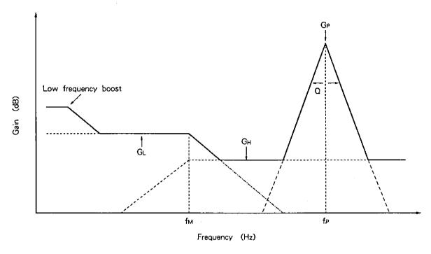
Fig. 2. Conceptual diagram of CXA1578 frequency characteristics
