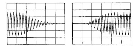
Fig. 4. Recording mute waveform
