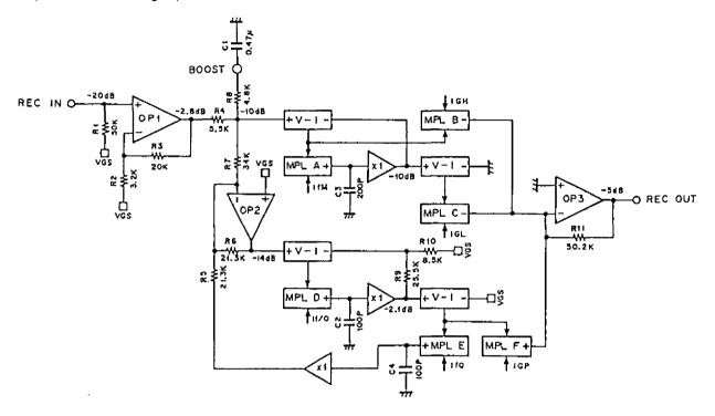
Fig. 1. CXA1578 functional circuit block diagram
