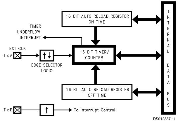
Note: The PWM output is not available in this mode since the TxA pin is being used as the counter input clock.
