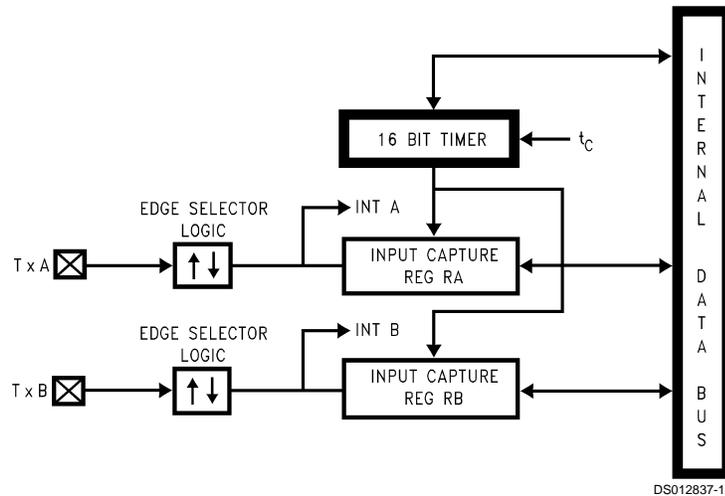
FIGURE 11. Timer in Input Capture Mode
