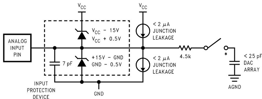
\*The analog switch is closed only during the sample time.
