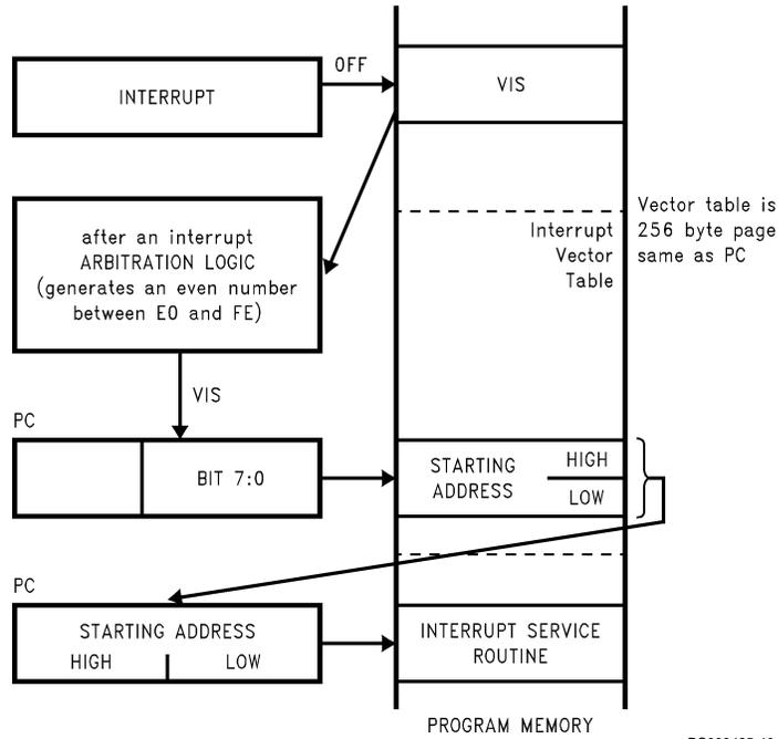
FIGURE 14. VIS Operation
