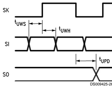
**FIGURE 3. MICROWIRE/PLUS Timing**
