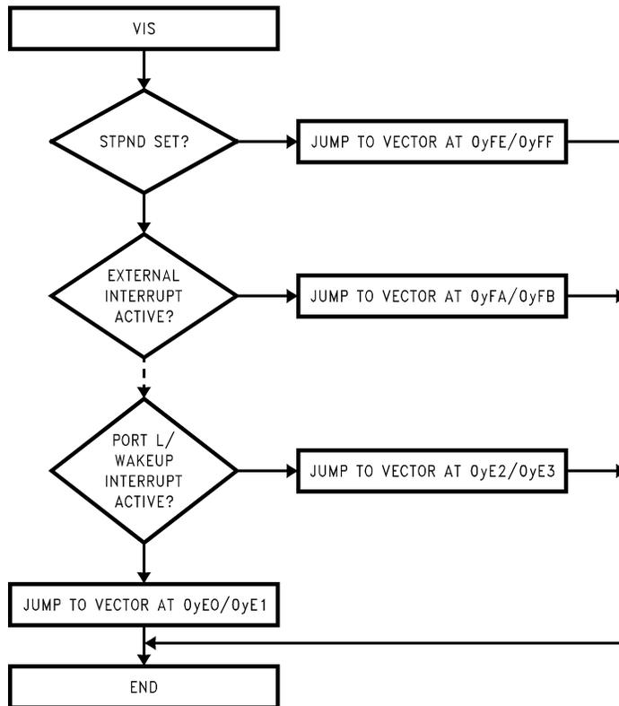
FIGURE 15. VIS Flowchart
