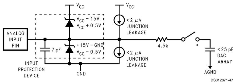
\* The analog switch is closed only during the sample time.
