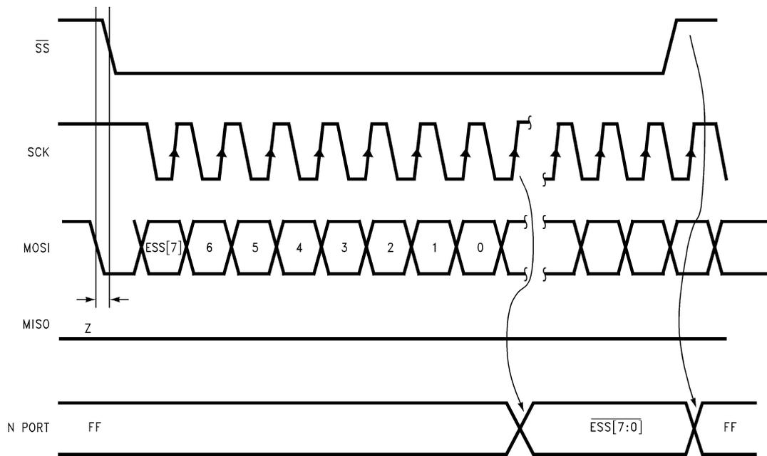
SESSEN = 1, SCE = 0. If MOSI = 0 at the falling edge of  $\overline{SS}$ , the  $\overline{ESS}$  programming mode is detected and all N-port alternate functions are enabled.
