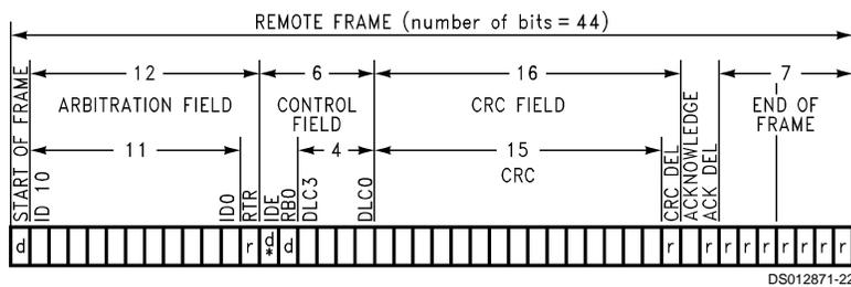
A remote frame is identical to a data frame, except that the RTR bit is "recessive", and there is no data field.
