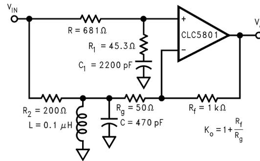
$$\frac{V_o}{V_{IN}} = K_o \left( \frac{sC_1R_1 + 1}{sC_1(R_1 + R) + 1} - \left( \frac{R_f}{R_f + R_g} \right) \frac{sLR_g}{s^2LCR_2R_g + sL(R_2 + R_g) + R_2R_g} \right)$$
