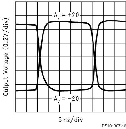
**Large Signal Pulse Response ( $V_O = 2V_{PP}$ )**
