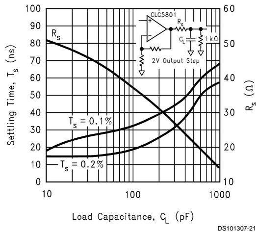
**Typical Performance Characteristics** ( $T_A = 25^\circ\text{C}$ ,  $V_{CC} = \pm 5\text{V}$ ,  $R_g = 26.1\Omega$ ,  $R_f = 499\Omega$ ,  $R_L = 100\Omega$ , unless otherwise specified).. (Continued)
