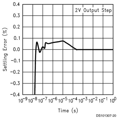
**Settling Time vs.  $C_L$  and  $R_S$**
