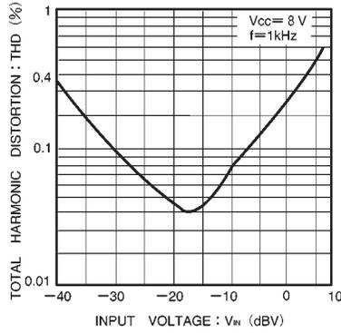
Fig. 6 Total harmonic distortion vs. input voltage
