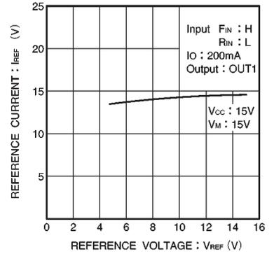
Fig.17  $V_{REF}$  reference current vs.  $V_{REF}$  reference voltage
