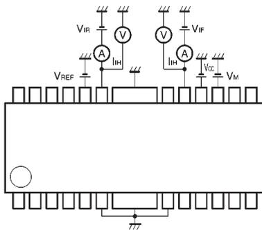
\* Refer to the truth table for output mode. HIGH and LOW level input voltages correspond to the readings of VIF and VIR voltmeters, respectively. The HIGH level input current is represented by the VIH ammeter reading when VIN = 2 V.
