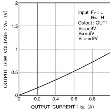
Fig.16 Output low level voltage vs. output current
