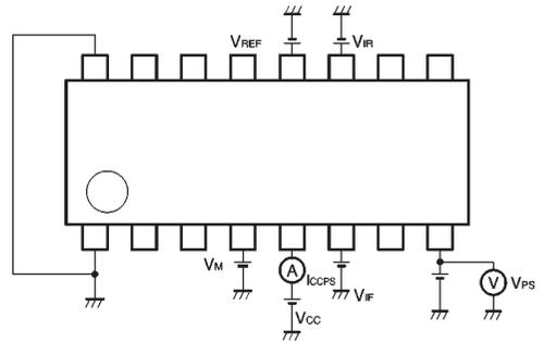
The power save mode ON voltage is represented by the  $V_{PS}$  reading when  $I_{CCPS}$  is  $15\ \mu\text{A}$  or less. The power save mode OFF voltage is represented by the  $V_{PS}$  reading when  $I_{CCPS}$  is more than  $15\ \mu\text{A}$ .
