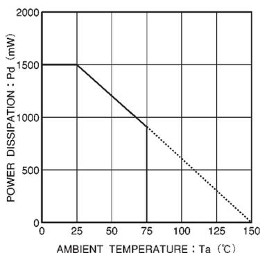
Fig.13 Temperature dependence of power dissipation curve (BA6285FP)
