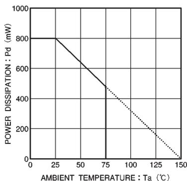
Fig.12 Temperature dependence of power dissipation curve (BA6285FS)
