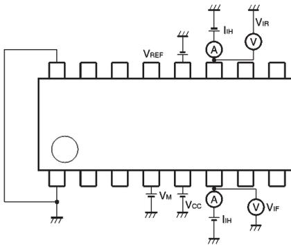
\* Refer to the truth table for output mode. HIGH and LOW level input voltages correspond to the readings of  $V_{IF}$  and  $V_{IR}$  voltmeters, respectively. The HIGH level input current is represented by the  $I_{IH}$  ammeter reading when  $V_{IN} = 2\text{ V}$ .
