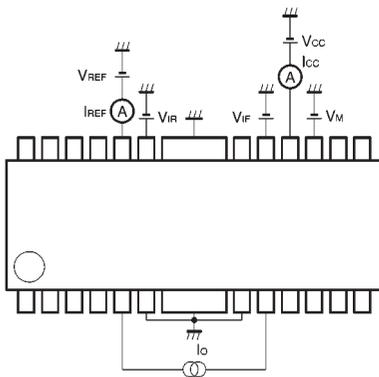
\* Refer to the truth table for output mode. The supply current is represented by the ICC-value, and the VREF sink current is represented by the IREF-value. The direction of the Io current is from the HIGH level to the LOW level output pin.
