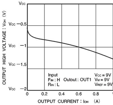
Fig.15 Output high level voltage vs. output current
