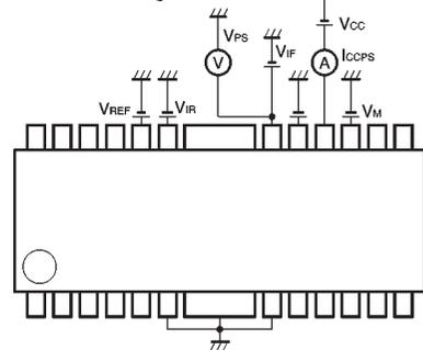
The power save mode ON voltage is represented by the VPS reading when ICCPS is 15 µA or less. The power save mode OFF voltage is represented by the VPS reading when ICCPS is more than 15 µA.
