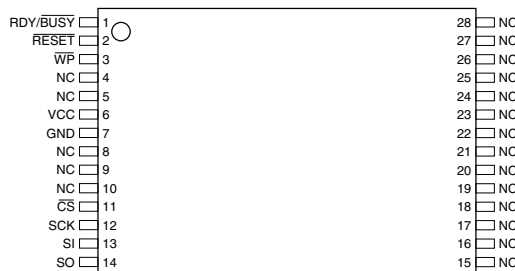
TSOP Top View Type 1
