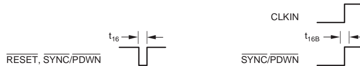
Figure 3. RESET and SYNC/PDWN Timing
