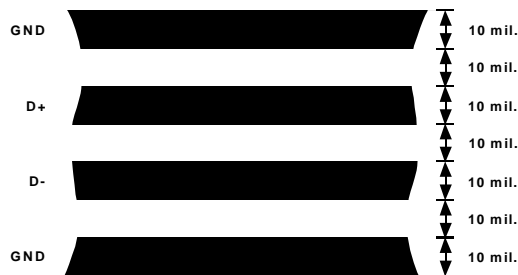
Figure 9. Arrangement of Signal Tracks
