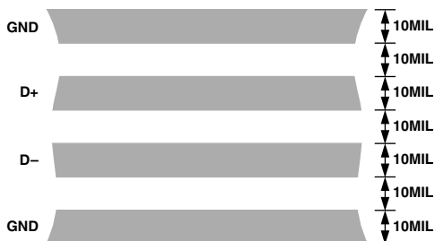
Figure 4. Arrangement of Signal Tracks
