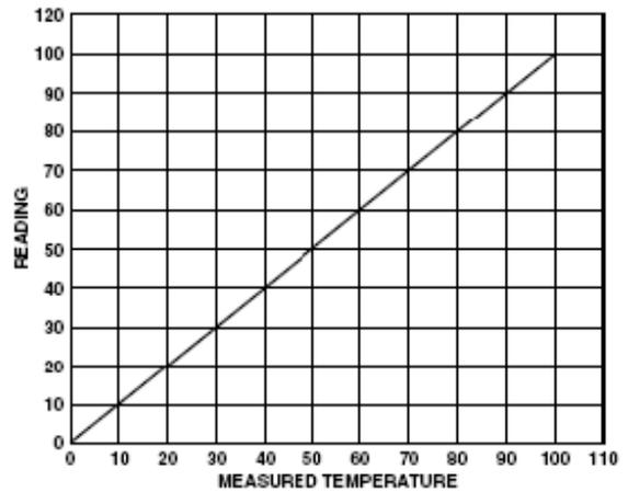
Figure 6. Pentium II<sup>®</sup> Temperature Measurement vs. ADM1025/ADM1025A Reading
