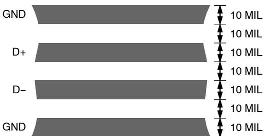
**Figure 15. Arrangement of Signal Tracks**
