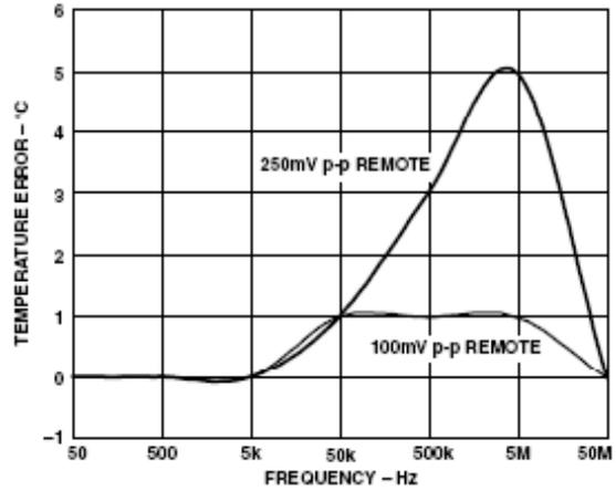
Figure 4. Temperature Error vs. Power Supply Noise Frequency
