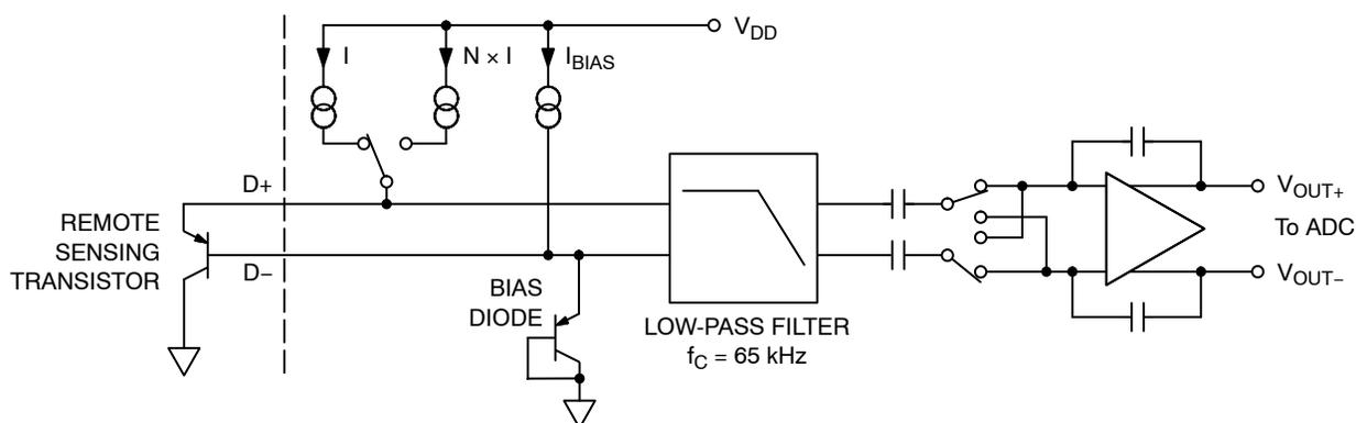
**Figure 14. Signal Conditioning for External Diode Temperature Sensors**
