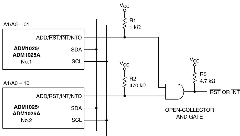
**Figure 16. Using Two ADM1025/ADM1025As on the Same Bus with a Common Interrupt**
