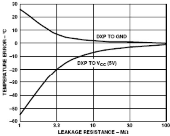
Figure 3. Temperature Error vs. PC Board Track Resistance
