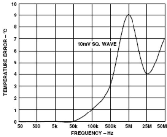
Figure 8. Temperature Error vs. Differential-mode Noise Frequency
