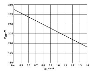
*Figure 26. Source Capability of Status Output* (ADDC02803SC)
