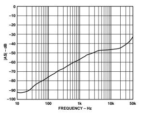
Figure 11. Audio Susceptibility (Magnitude of  $V_{OUT}/V_{IN}$ ) (ADDC02805SA)
