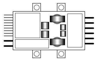
Figure 34. Hot Spots (Shaded Areas) of DC/DC Converter
