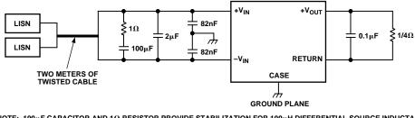
NOTE: 100μF CAPACITOR AND 1Ω RESISTOR PROVIDE STABILIZATION FOR 100μH DIFFERENTIAL SOURCE INDUCTANCE INTRODUCED BY THE LISNS. REFER TO SECTION ON EMI CONSIDERATIONS FOR MORE INFORMATION.
