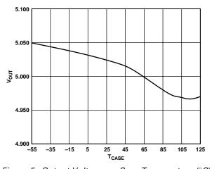
Figure 5. Output Voltage vs. Case Temperature (°C) (ADDC02805SA)
