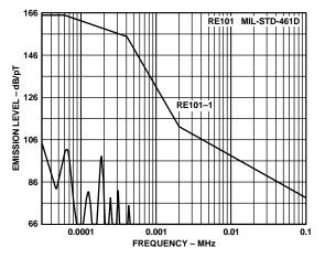
Figure 21. Radiated Emissions, MIL-STD-461D, RE101, 100 W Load
