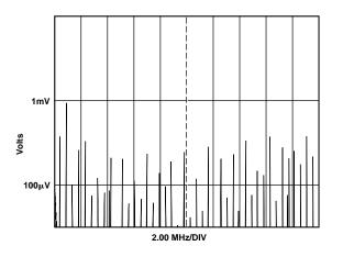
*Figure 18. Output Voltage Ripple Spectrum* (ADDC02805SA)
