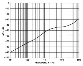
Figure 12. Audio Susceptibility (Magnitude of  $V_{OUT}/V_{IN}$ ) (ADDC02803SC)
