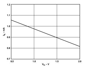
Figure 31. Input Characteristics of Pin 6 When Pulled Low
