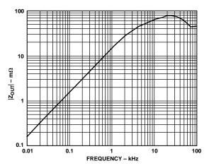
Figure 15. Incremental Output Impedance (Magnitude) (ADDC02805SA)
