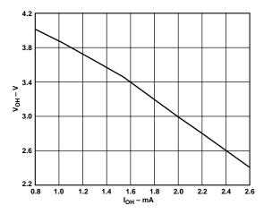
Figure 27. Source Capability of Status Output (ADDC02805SA)
