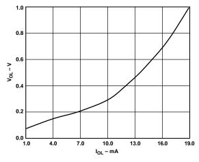
Figure 28. Sink Capability of Status Output
