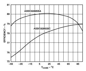
Figure 3. Efficiency vs. Case Temperature (°C) (at Nominal V<sub>IN</sub>, 75% Max Load)
