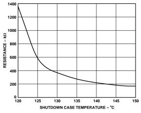
Figure 32. External Resistor Value for Raising Temperature Shutdown Point
