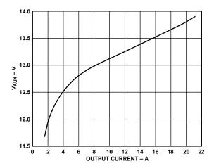
*Figure 30. V*<sub>AUX</sub> *vs. Converter Output Current* (ADDC02803SC)
