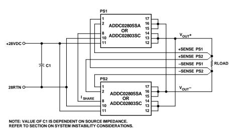
Figure 37. Typical Connections for Paralleling Two Converters
