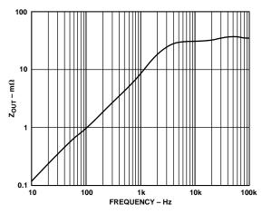
Figure 16. Incremental Output Impedance (Magnitude) (ADDC02803SC)
