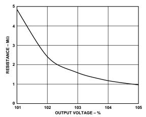
Figure 25. External Resistor for Increasing Output Voltage
