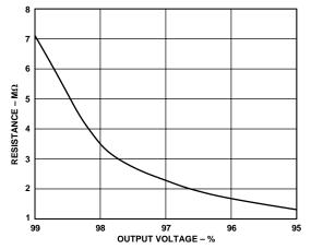
Figure 24. External Resistor Value for Reducing Output Voltage
