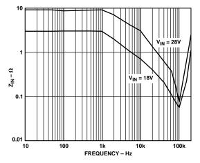
Figure 14. Incremental Input Impedance (Magnitude) (ADDC02803SC)
