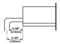
Figure 35. Minimum Bend Radius of 40 Mil (1.02 mm) Pins
