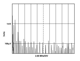
Figure 17. Output Voltage Ripple Spectrum (ADDC02803SC)
