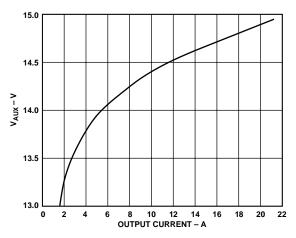
*Figure 29. V<sub>AUX</sub> vs. Converter Output Current* (*ADDC02805SA*)
