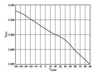
Figure 6. Output Voltage vs. Case Temperature (°C) (ADDC02803SC)
