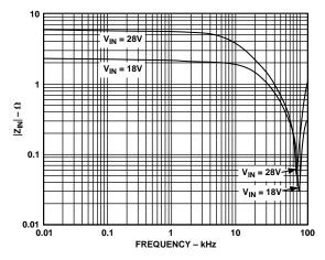
*Figure 13. Incremental Input Impedance (Magnitude) (ADDC02805SA)*
