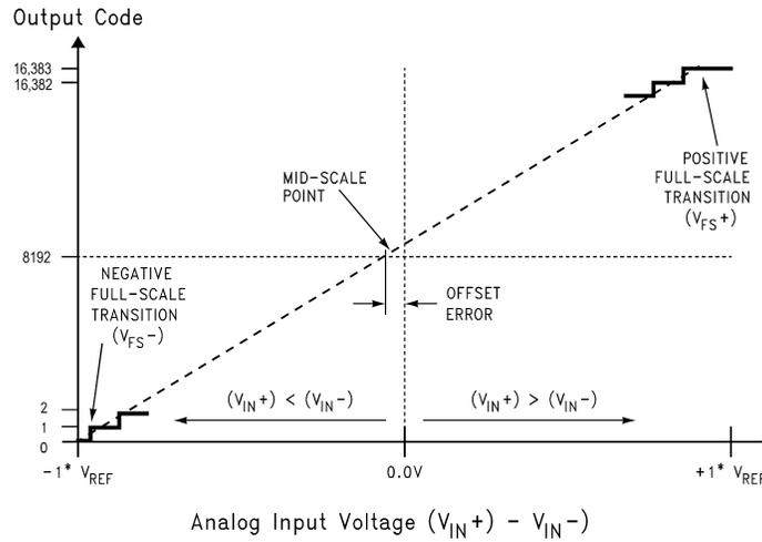
**Figure 2. Transfer Characteristic**
