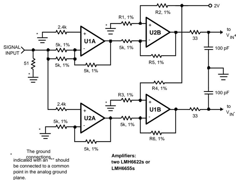
Figure 37. Differential Drive Circuit of Figure 36
