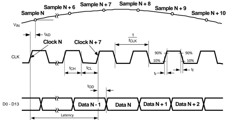
Figure 1. Output Timing
