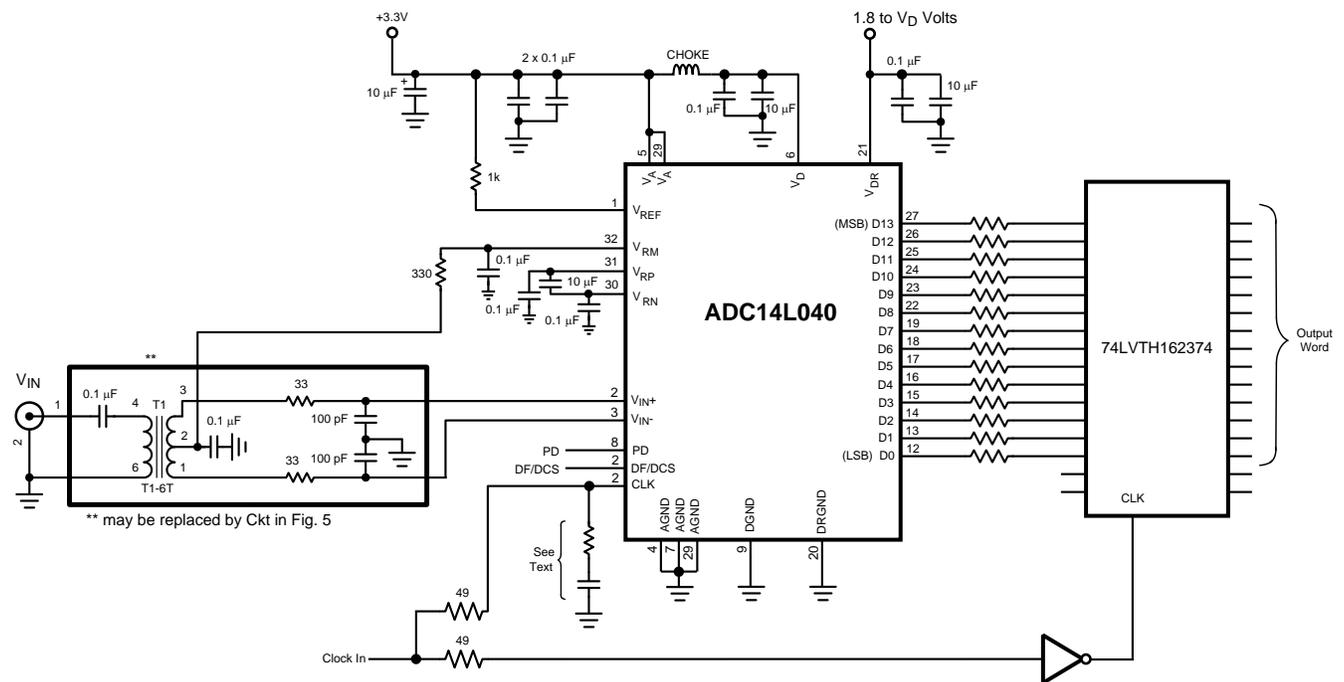
**Figure 36. Application Circuit using Transformer Drive Circuit**
