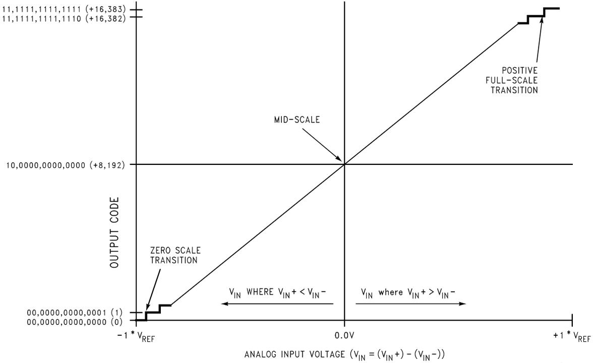
FIGURE 1. Transfer Characteristic
