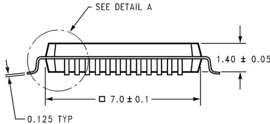
**48-Lead TQFP Package**
