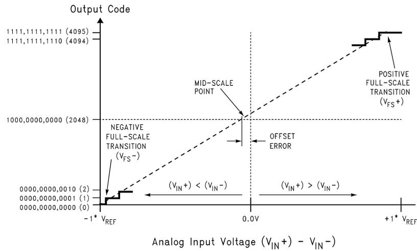
**Figure 4. Transfer Characteristic**
