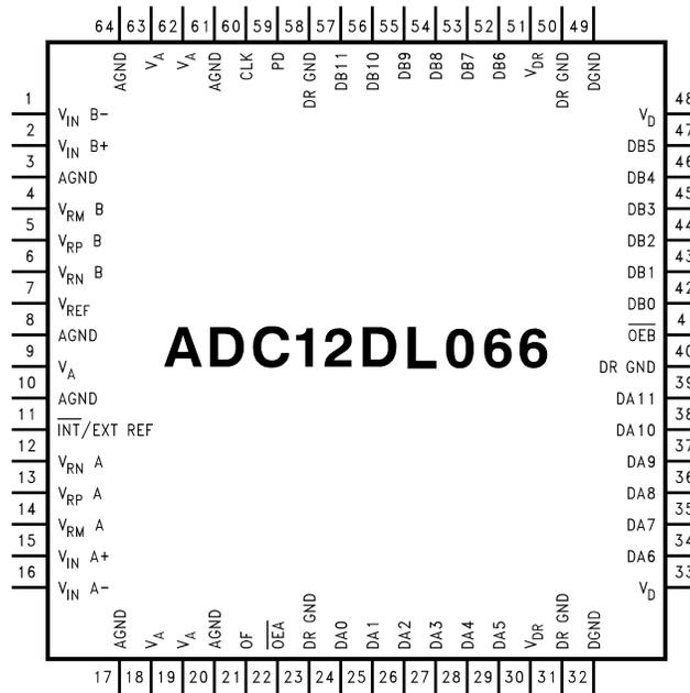
Figure 1. 64-Lead TQFP Package
