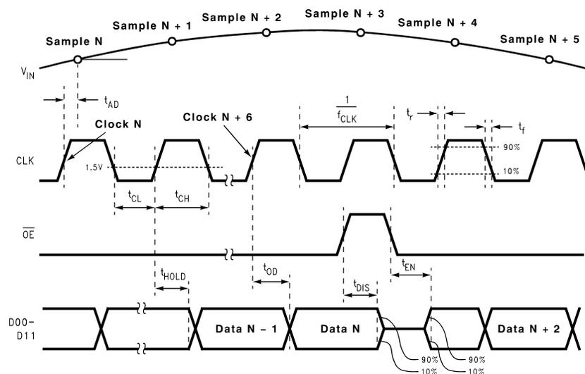
**Figure 3. Output Timing**
