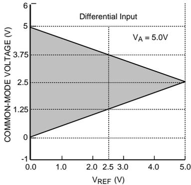
Figure 46.  $V_{CM}$  range for Differential Input operation
