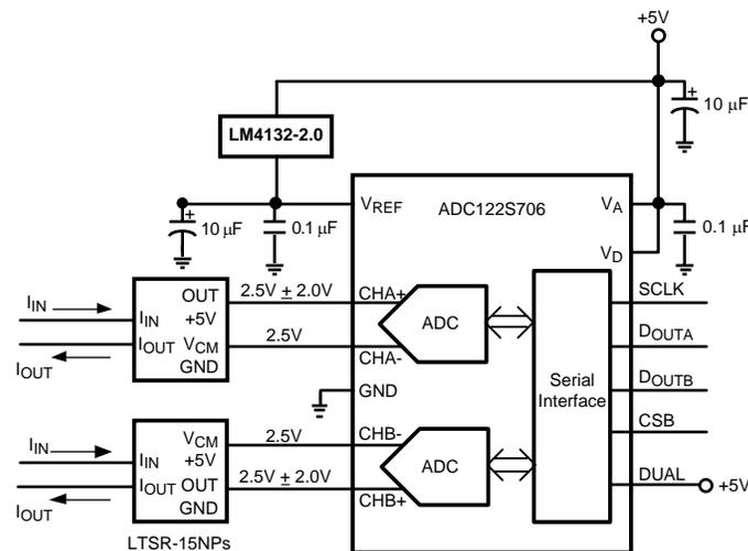
Figure 49. Interfacing the ADC122S706 to a Current Transducer
