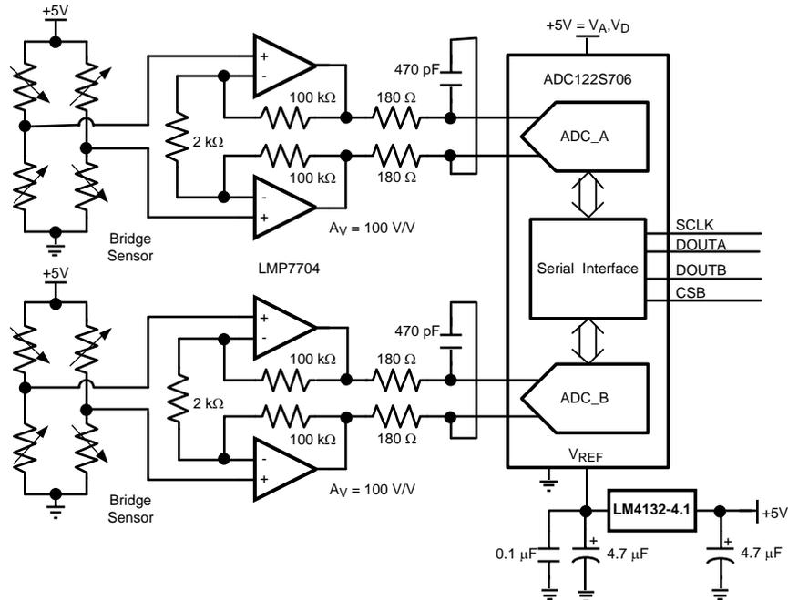
Figure 50. Interfacing the ADC122S706 to Bridge Sensors
