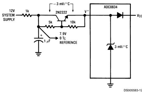
FIGURE 4. Operating with a Temperature Compensated Reference
