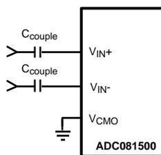
**Figure 34. Differential Input Drive**
