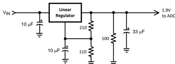
**Figure 38. Non-Spiking Power Supply**
