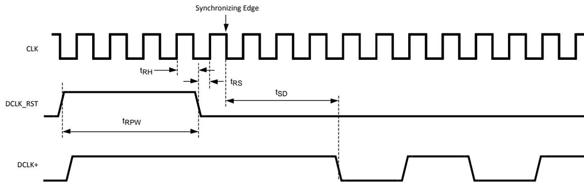
Figure 5. Clock Reset Timing in DDR Mode
