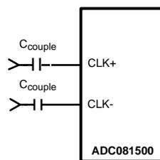
**Figure 37. Differential (LVDS) Input Clock Connection**
