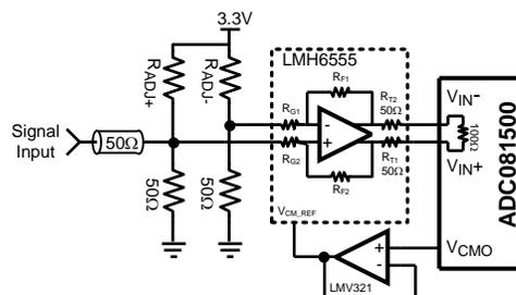
**Figure 36. Example of Servoing the Analog Input with  $V_{CMO}$**
