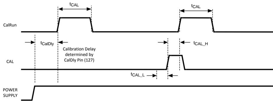
**Figure 8. Self Calibration and On-Command Calibration Timing**
