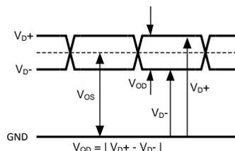
**LVDS OUTPUT OFFSET VOLTAGE ( $V_{OS}$ )** is the midpoint between the D+ and D- pins output voltage; i.e.,  $[(V_{D+}) + (V_{D-})]/2$ .
