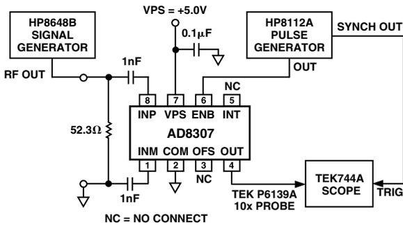
TPC 15. Test Setup for Power-Up/Power-Down Response Time
