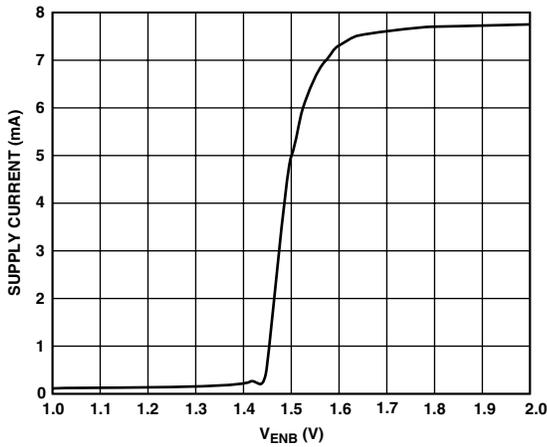
TPC 2. Supply Current vs.  $V_{ENB}$  Voltage (3 V)
