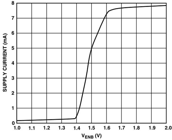
TPC 1. Supply Current vs.  $V_{ENB}$  Voltage (5 V)
