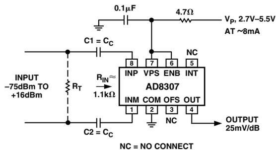
Figure 12. Basic Connections
