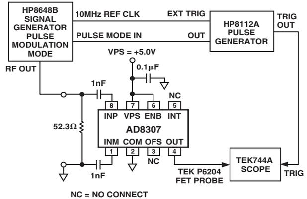
TPC 18. Test Setup for  $V_{OUT}$  Pulse Response
