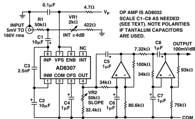
Figure 20. Log Amp with Four-Pole Low-Pass Filter
