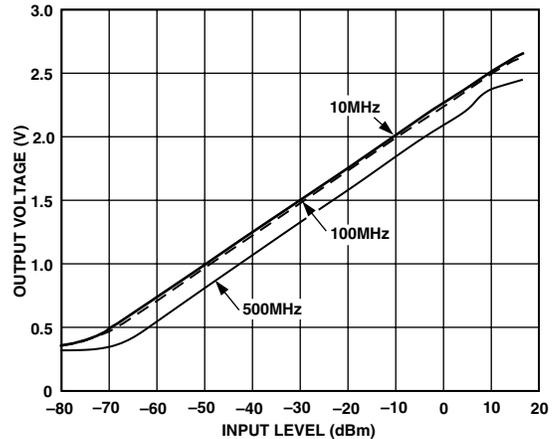
Figure 13. Log Response at 10 MHz, 100 MHz, and 500 MHz
