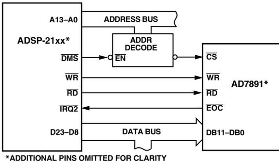
Figure 12. AD7891 to ADSP-21xx Parallel Interface
