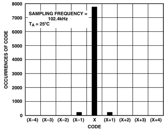
Figure 19. Histogram of 8192 Conversions with Write During Conversion
