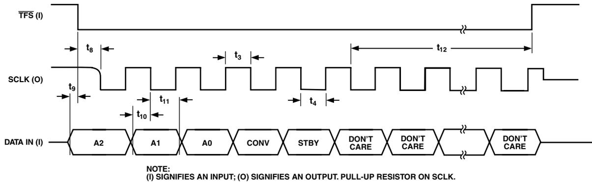
Figure 9. Self-Clocking (Master) Mode Control Register Write
