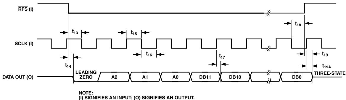
Figure 10. External Clocking (Slave) Mode Output Register Read
