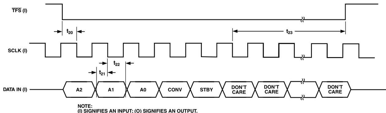
Figure 11. External Clocking (Slave) Mode Control Register Write
