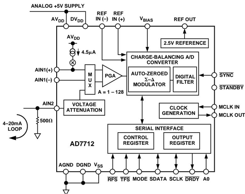
Figure 21. 4–20 mA Loop Measurement Using the AD7712
