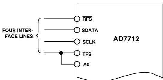
Figure 15. Simplified Interface with  $\overline{\text{TFS}}$  Connected to A0
