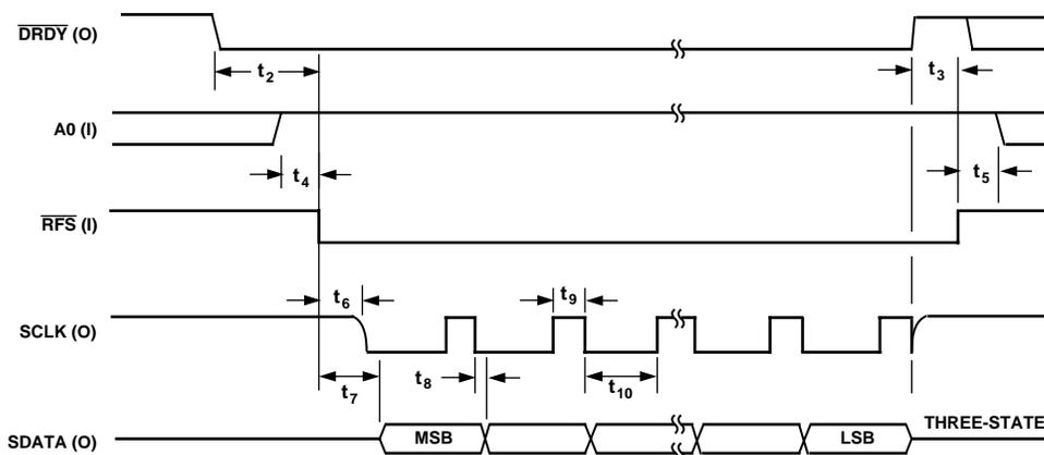
Figure 11. Self-Clocking Mode, Output Data Read Operation
