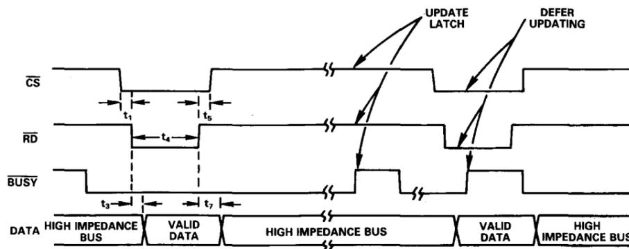
Figure 9. Asynchronous Conversion Mode Timing Diagram
