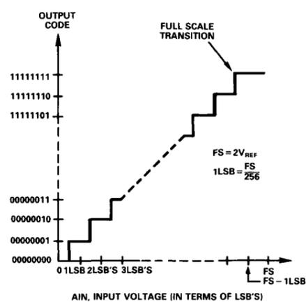
Figure 4. Nominal Transfer Characteristic for Unipolar Operation
