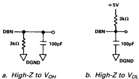
Figure 1. Load Circuits for Data Access Time Test
