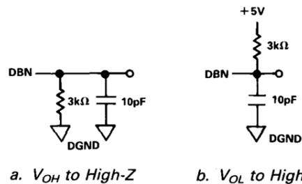
Figure 2. Load Circuits for Data Hold Time Test
