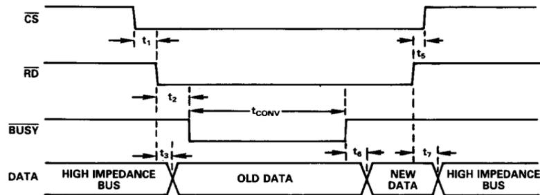
Figure 5. Slow Memory Interface Timing Diagram
