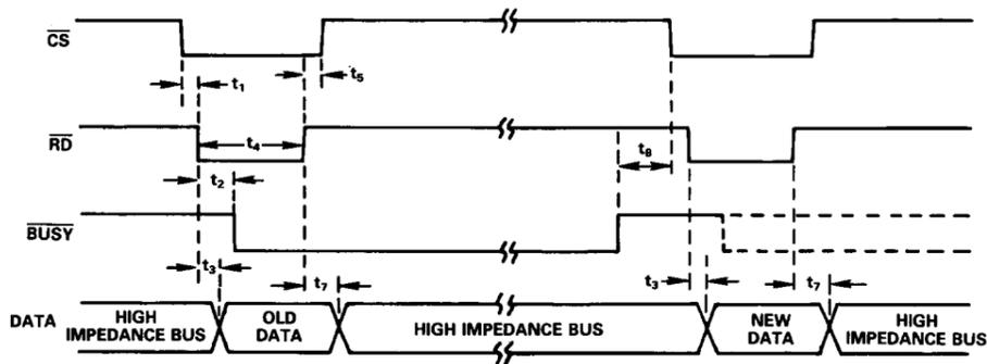
Figure 7. ROM Interface Timing Diagram
