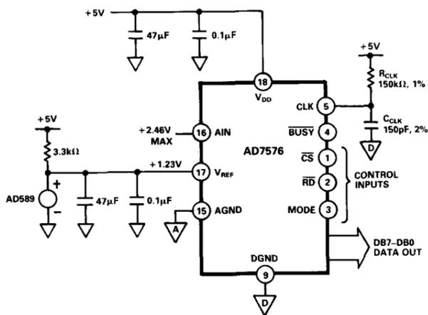
Figure 3. AD7576 Operational Diagram
