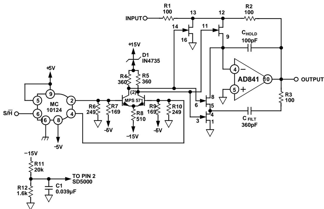
Figure 27. High Performance, Low Cost Deglitching Circuit
