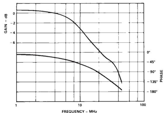
Figure 17. Large Signal Gain and Phase Response
