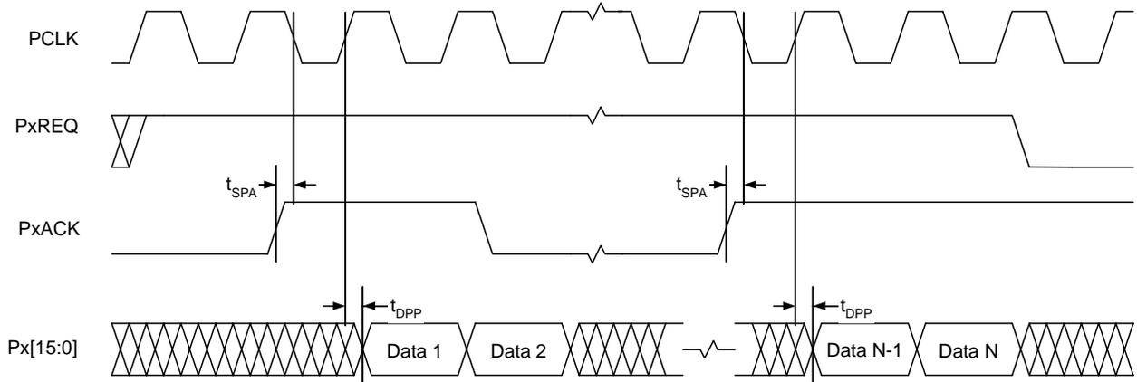
Figure 13. Slave Mode PxACK to PCLK Switching Characteristics
