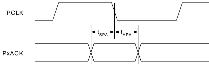
Figure 9. Master Mode PxACK to PCLK Setup and Hold Characteristics
