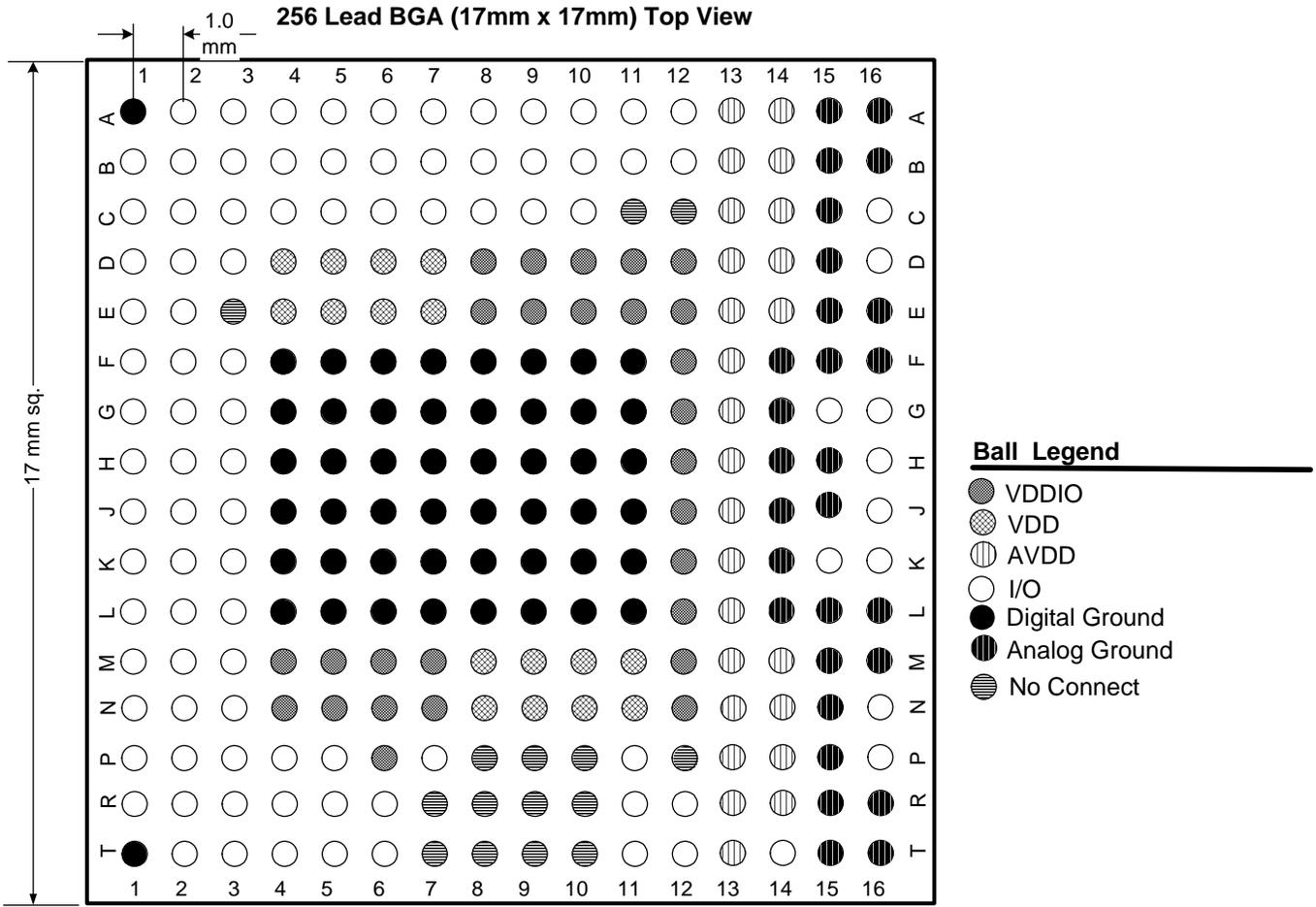
Figure 2. 17 x 17 Mini-BGA package showing power and signal ball assignments
