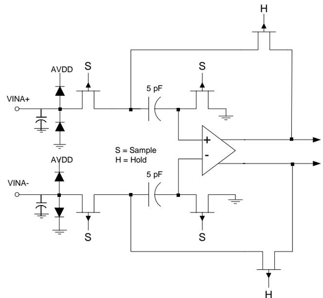
Figure 22. Switched-Capacitor SHA Input for one ADC channel
