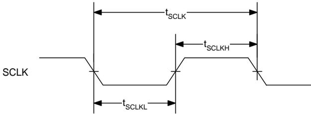
Figure 43. SCLK Timing Requirements
