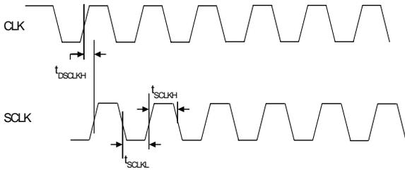
Figure 44. SCLK Switching Characteristics (Divide by 1)
