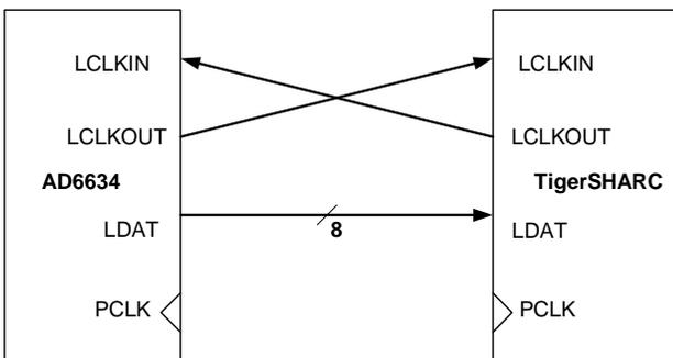
Figure 39. Link Port Connection Between AD6652 and TigerSHARC
