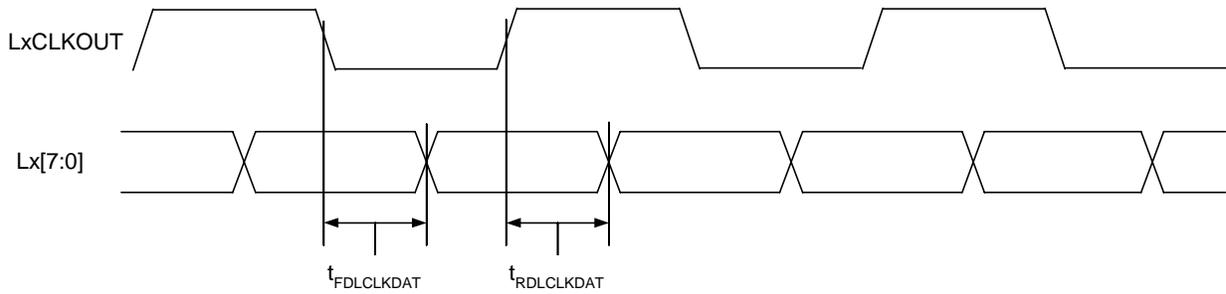
Figure 17. LxCLKOUT to Lx[7:0] Data Switching Characteristics
