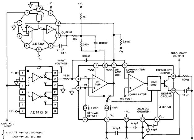
Figure 13. Auto-Zero Circuit for AD650 Voltage-to-Frequency Converter
