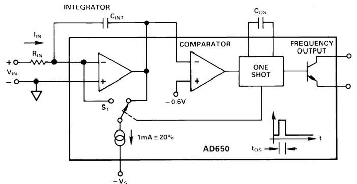
Figure 2a. Block Diagram
