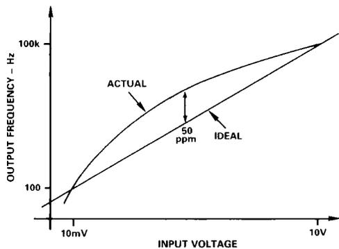
Figure 9a. Exaggerated Nonlinearity at 100 kHz Full Scale
