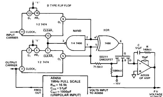
Figure 14. Phase Locked Loop F/V Conversion
