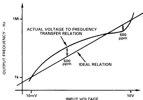
Figure 9b. Exaggerated Nonlinearity at 1 MHz Full Scale
