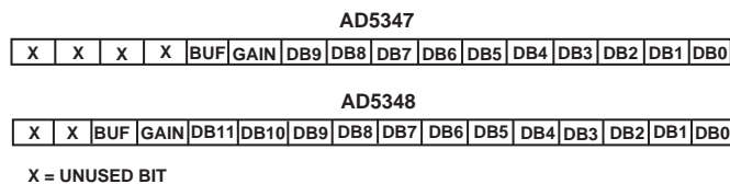
Figure 10. AD5347/AD5348 Data Format for Word Load with GAIN and BUF Data on 16-Bit Bus
