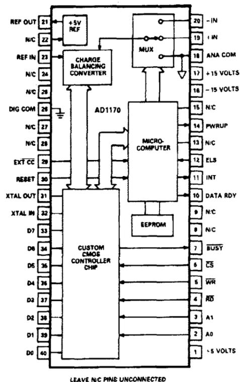
2. The AD1170 architecture provides for user programmable data format independent of the integration time. All data is computed to 22-bit resolution and the user may specify any resolution from 7 to 22 bits. Usable resolution will typically be limited to 18-bits due to measurement and calibration noise error.
