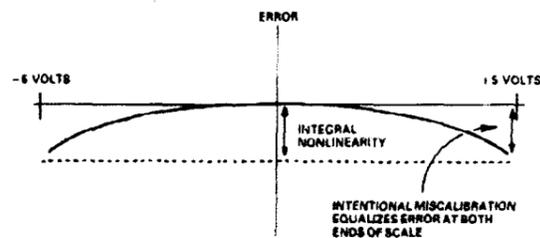
Figure 3. Relative Accuracy with Intentional Span Error at +F.S.
