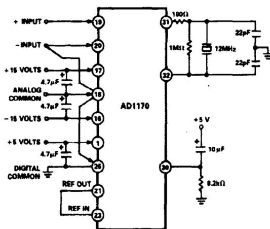
Figure 5. Input, Power, Reset, and Clock Connections
