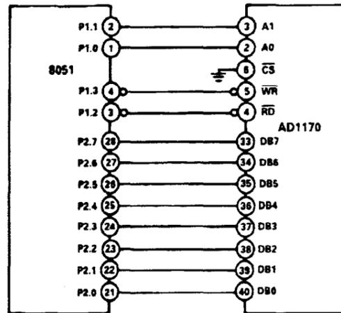
Figure 13. Simple 8051 to AD1170 Interface
