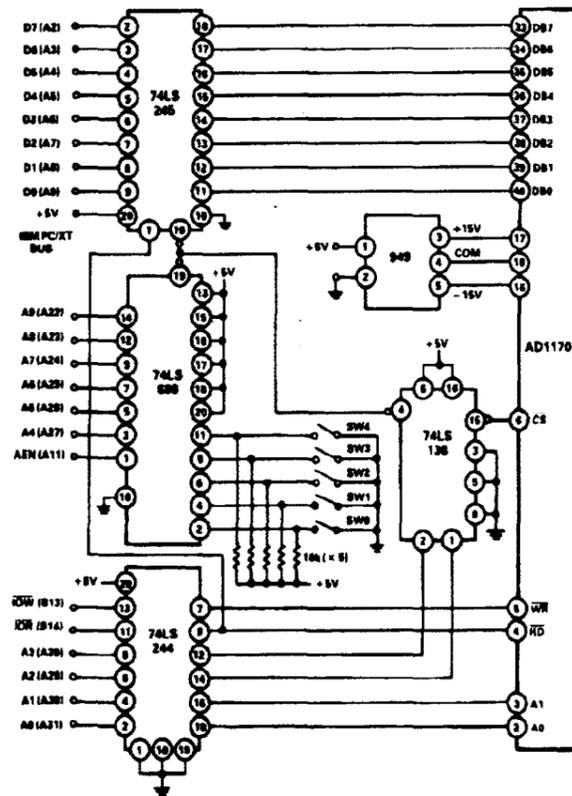
Figure 12. IBM PC/XT to AD1170 Interface
