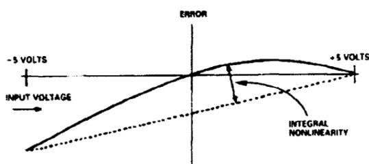
Figure 2. Relative Accuracy and Integral Nonlinearity when Calibrated
