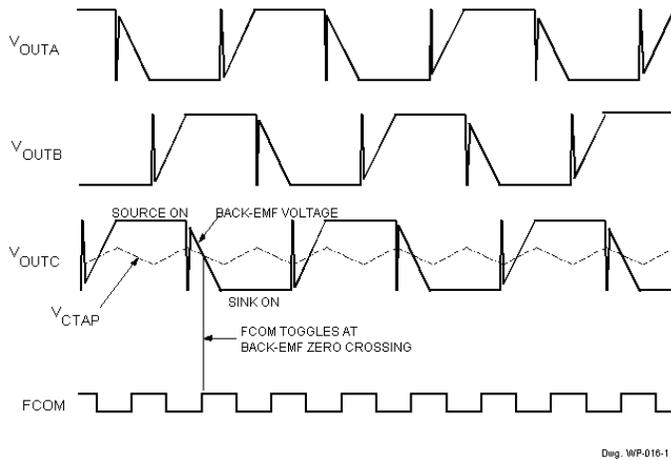
True back-EMF zero crossings are used by the adaptive commutation delay circuit to advance the state sequencer (commutate) at the proper time to synchronously run the motor. See next section.
