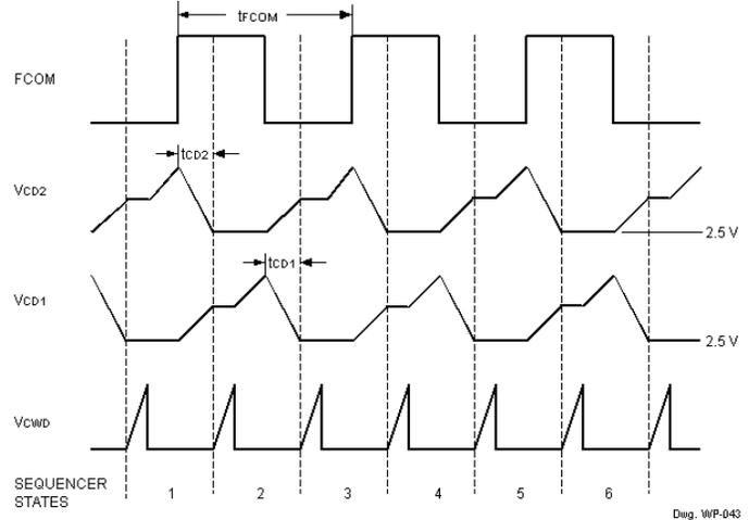
The typical delta voltage change during normal operation in the commutation capacitors ( $C_{D1}$  &  $C_{D2}$ ), will range between 1.5 V and 2.0 V. The commutation capacitor values can be determined from:
