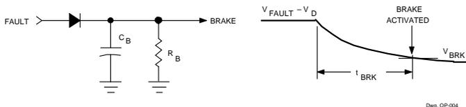
The brake delay can be set using the equation:
