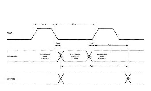
Note: All times measured from 50% points, for all input waveforms tr =  $t_f$ <10nsec.
