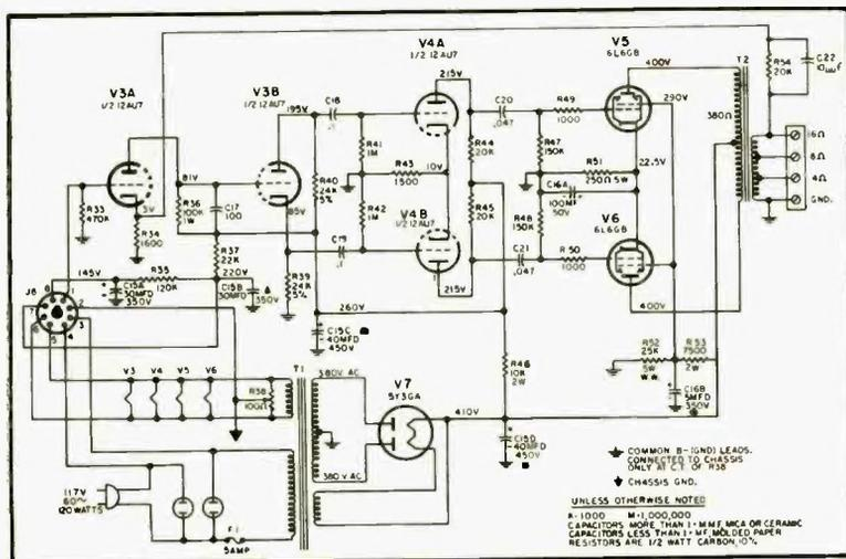
Fig. 4. Schematic of the power amplifier section.
