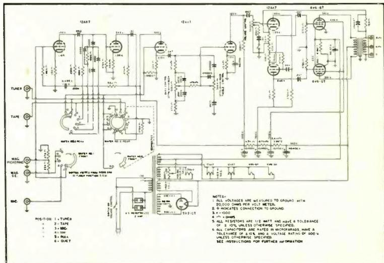
Fig. 9. Over-all schematic for the Rauland 1811 Amplifier.
