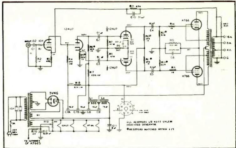
Fig. 5. Schematic of the UL-1 power amplifier.
