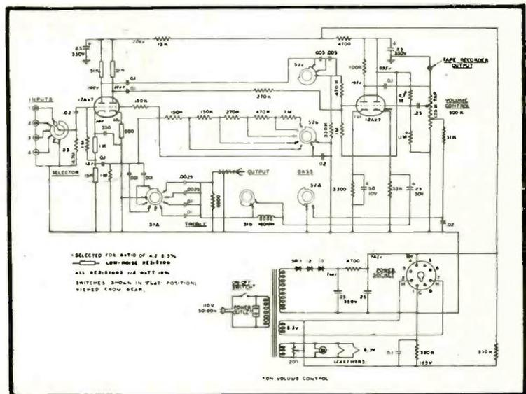
Fig. 6. Schematic of the CA-2 control amplifier.
