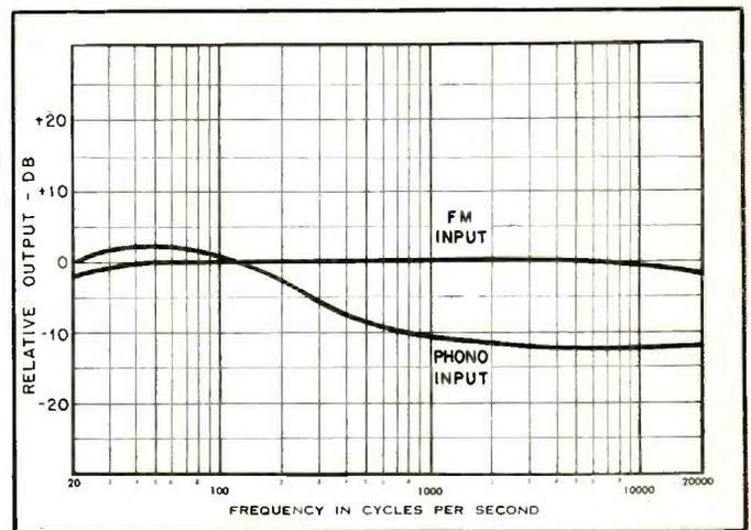
series-resonant circuit; the rise in gain after the frequency of maximum attenuation is due to the inability of the series-resonant circuit to keep the response down. The results are quite satisfactory despite these peaks, and in spite of the grave admonitions to avoid peaks, the "ringing" of the system is not noticeable to the listener.
